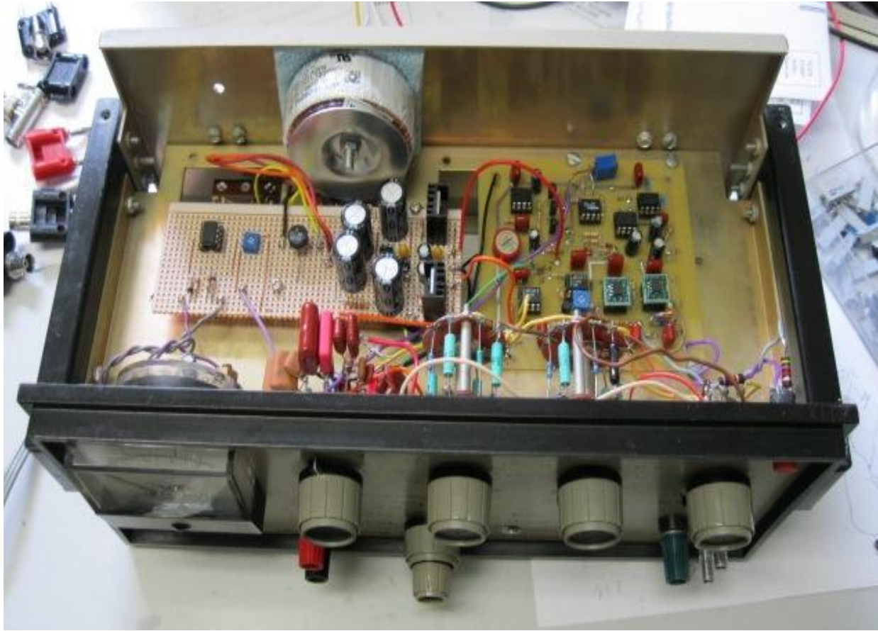
Top view of the oscillator, showing the osc. board, right, and the power supply & meter board, left. The toroid power transformer is on the back panel (see the bottom of the page for an important change in location). If you use the Heath power transformer, there's still room for a power supply/meter amp board in the chassis. Note the two OPA1641 on the adapters at bottom-right of the board.
